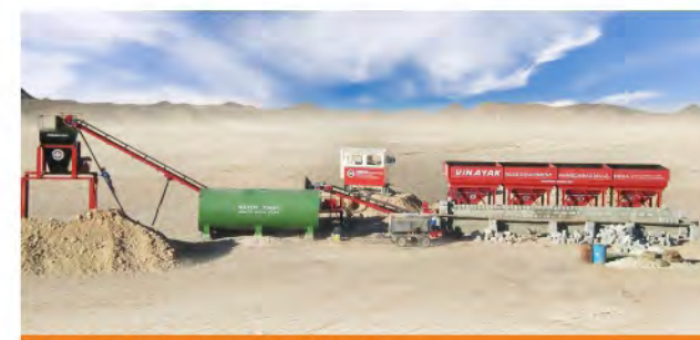
Wet Mix Macadam Plant
